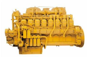
Cat 3516 engines set the standard in the drilling industry. For many years the 3500 has been the preferred choice by drillers due to their high performance, durability, and reliability in the oilfield. The ideal application for the 3512 engine is mechanical drive for land drilling rigs. 3516 engines, with ratings: 1230 bkW (1649 bhp) @ 1200 rpm. Not emissions certified, available for non-regulated areas.
